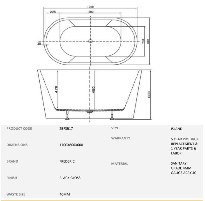
Please note that these dimensions will vary by a few millimeters and DRJ ASTRALIA PTY LTD is not liable if the installer uses the specifications to rough in, this is only a guide only. DRJ advises to have the DRJ product onsite when roughing in, this will assure the job is done correctly and accurately. Any information in regards to installation, please contact DRJ AUSTRALIA PTY LTD on:
